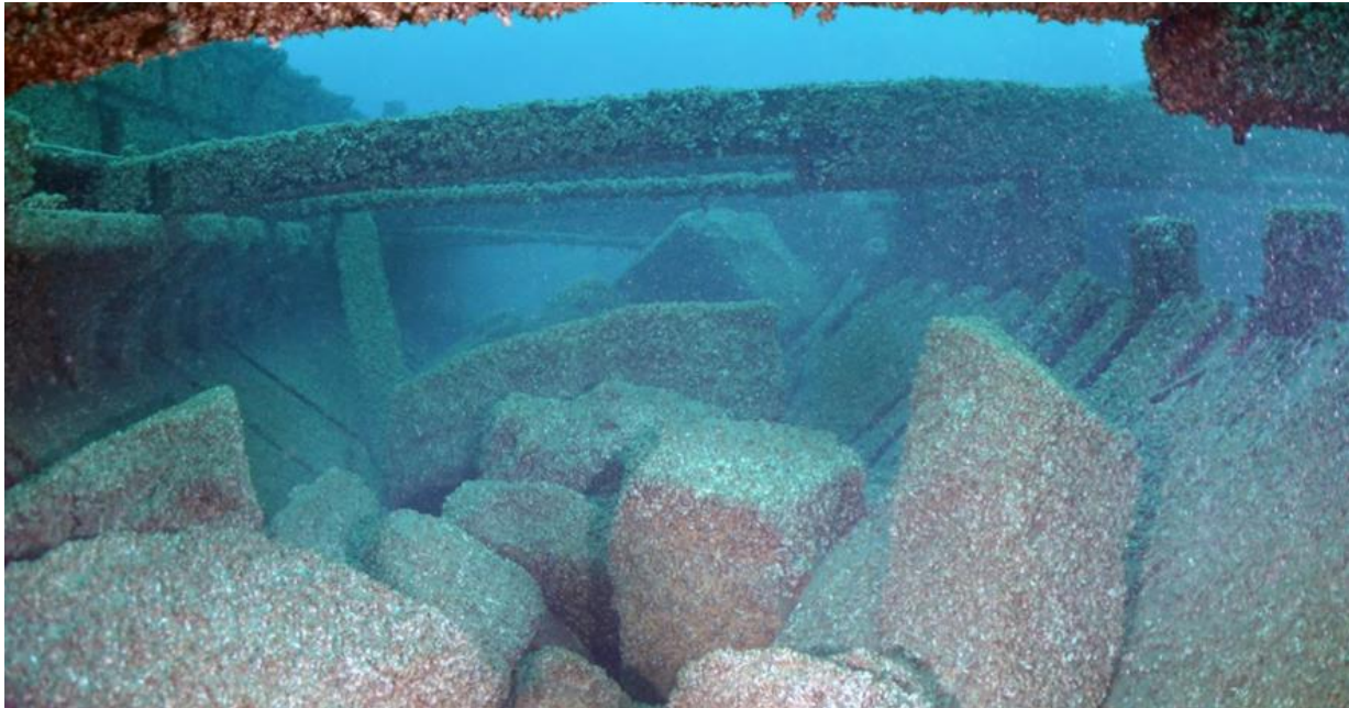
Figure 57. The upper portion of EMBA 's hoppers showing tie rods extending across the hold, and the removed deck planking (Wisconsin Historical Society)
