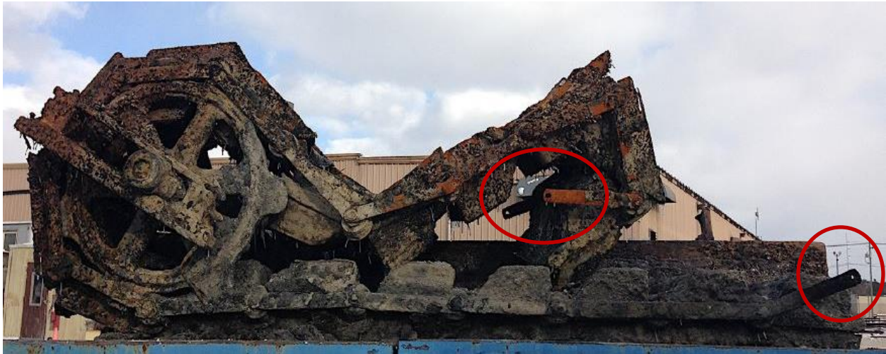
Figure 41. The 18 pan conveyor buckets after recovery. Note the evidence of dismantling and salvage (PanAmerican Consultants)
