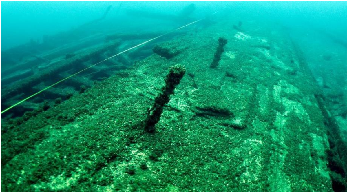
Figure 51. Transfer 's tie rods extending through the port side hull (Wisconsin Historical Society)
