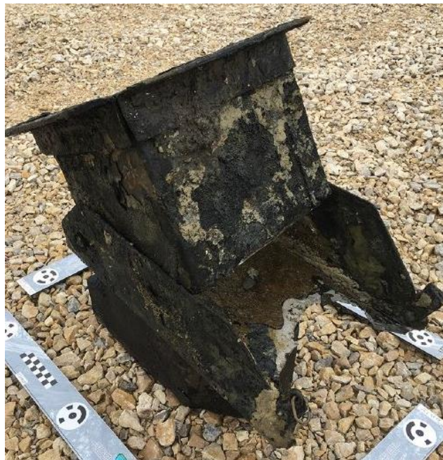
Figure 38. A hopper chute door recovered from Adriatic (PanAmerican Consultants)
