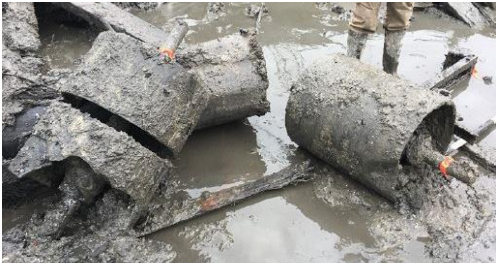
Figure 9. Two large belt conveyor rollers and a tensioner recovered from the Adriatic shipwreck (PanAmerican Consultants, Inc.)
