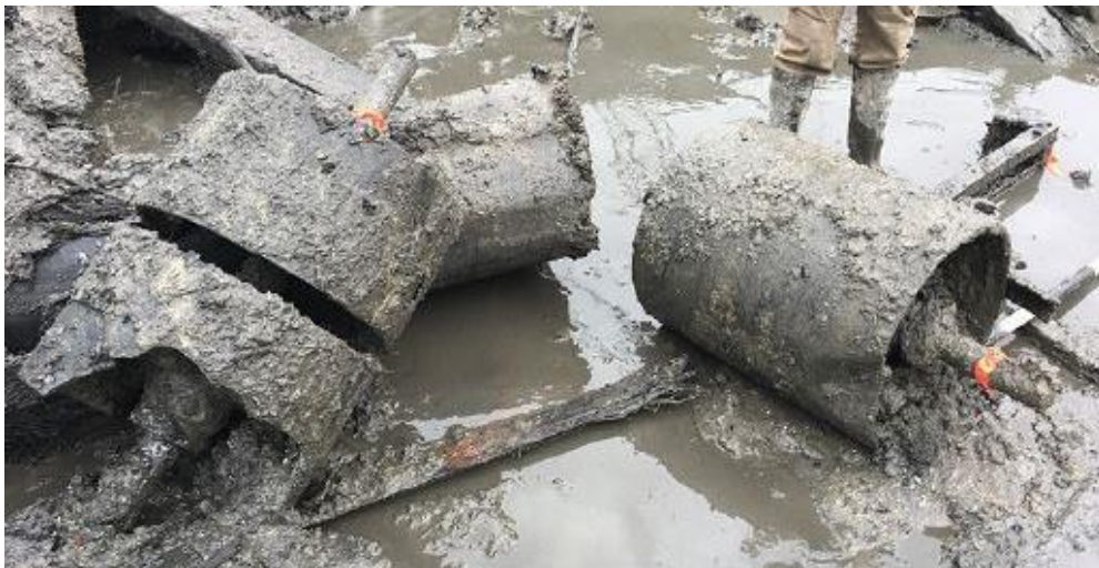
Figure 36. Two large belt conveyor rollers and tensioner recovered from the Adriatic shipwreck (PanAmerican Consultants)
